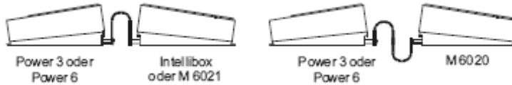
Figure 2.41. Orientation of the flat ribbon cable between Power 3/6 and different central units.
